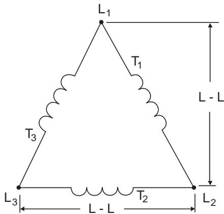
Three lead generators have 3 coil groups with one end of each group connected into a Delta internally. There are 3, 6, or 12 cables or 3 bus bars coming out of the generator.
