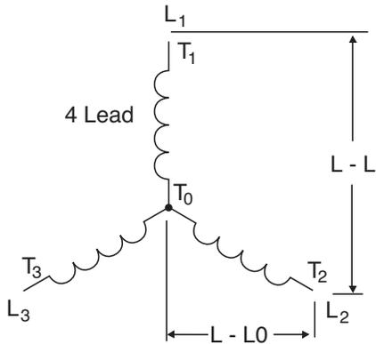
Four lead generators have 3 coil groups with one end of each group connected together. There are 4, 8, or 16 cables or 4 bus bars coming out of the generator.
