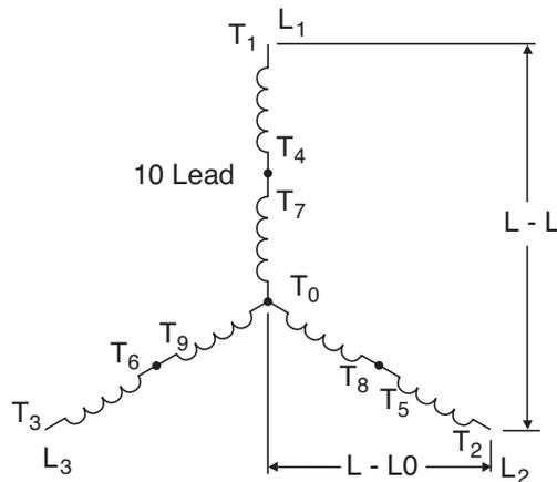
Ten lead generators are dual voltage generators with six coils. One end of the three inner coils is connected together. There are 10 or 20 cables coming out of the generator.
